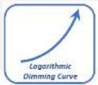
Logarithmic curve, close to human vision, providing comfortable dimming experience
